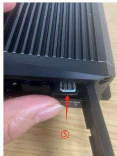
④Place the SIM card into the card tray in the direction of the silkscreen logo.
