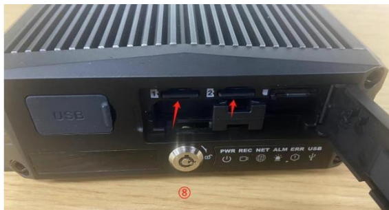
⑦ Insert the card into the Micro SD card slot in the direction shown in the illustration
