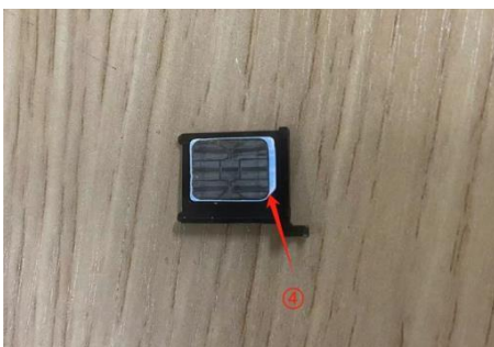
④Place the SIM card into the card tray in the direction of the silkscreen logo.
