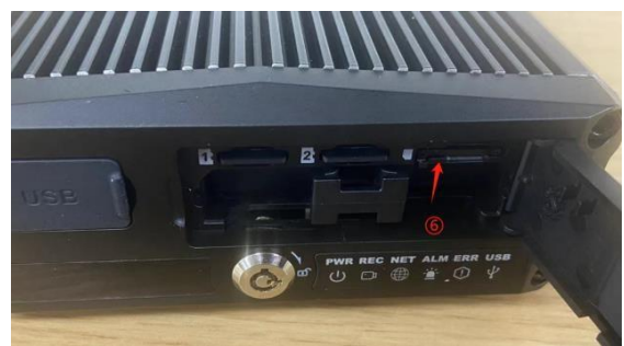
④Place the SIM card into the card tray in the direction of the silkscreen logo.
