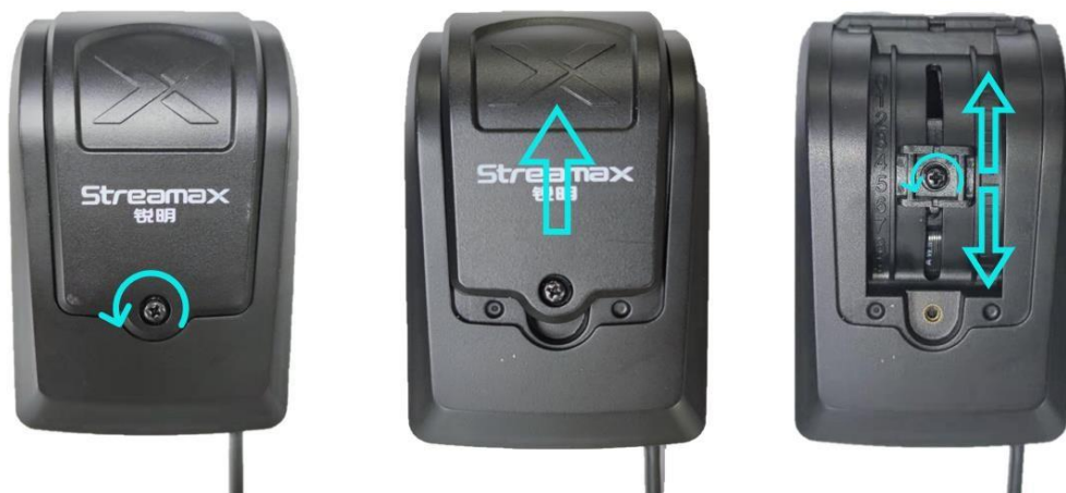
Dismantle the screw Remove the back cover Unscrew the screw and adjust the lens
