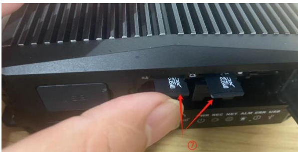
⑦ Insert the card into the Micro SD card slot in the direction shown in the illustration
