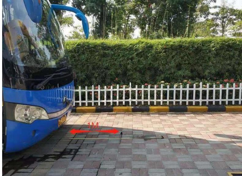
2 ) Adjust the angle of the camera so that the 1 meter calibration line coincides with the lower edge on the video screen, this calibration will achieve the correct tilt angle for the C20D wide angle lens.
