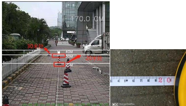
5) Adjust the camera angle, make the 20-meter calibration line match the object placed on the O&M screen, this will adjust the tilt angle of the C20D telephoto lens.
