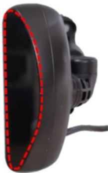
Left A-pillar installation: curved surface facing the cabin, wire end facing down.
