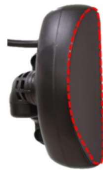
Right A-pillar installation: curved surface facing the cabin, wire end facing up.
